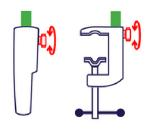
2. Insert arm into peg or clamp and tighten flower screw.
