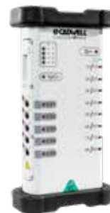
The IOMAX Limb Module is designed for recording and stimulating the arms and legs
