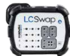
LCSwap is a comprehensive switch matrix solution for direct cortical stimulation
